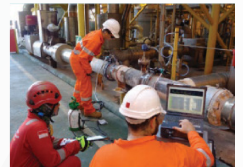
Sonomatic inspectors carrying out Chime Inspection
