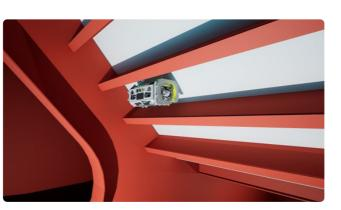
i-COT is seen not as one tool but as the delivery tool for a suite of un-manned and robotic Advanced NDT methods, each of which is selected specific to the inspection requirements of the tank.
